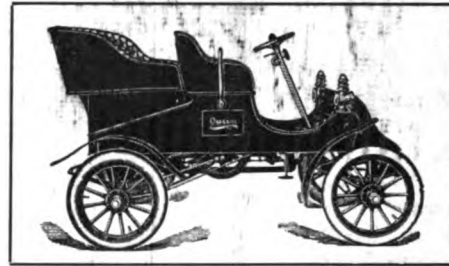
Model B. Touring Car. 12 Horse-power two cylinder opposed type.
